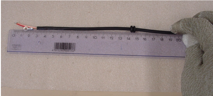
Fig. 3-6 Take the new power cable assy and slide the black wire tulle (item 06.2) to 14.5 cm
